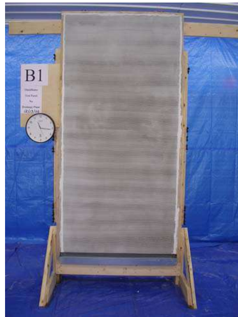
Figure 45: Panel B surface, 21 hours after spray application #1
