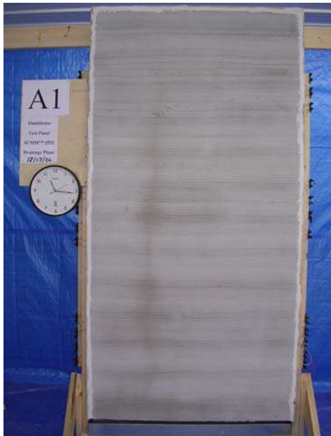
Figure 44: Panel A surface, 21 hours after spray application #1
