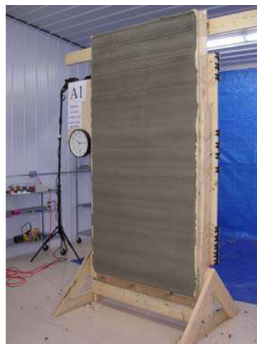
Figure 39: Scratch coat completed
