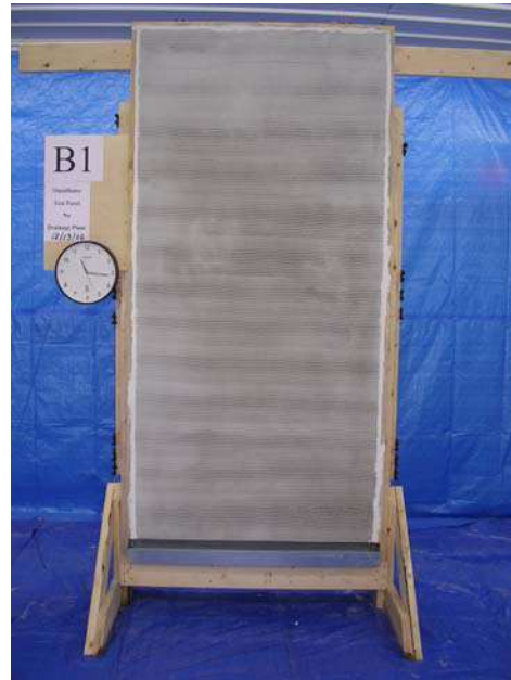
Figure 45: Panel B surface, 21 hours after spray application #1
