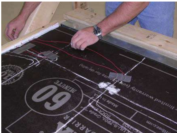
Figure 14: Affixing sensor wires
