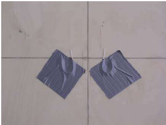
Figure 3: Plywood Layer sensor contact points.
