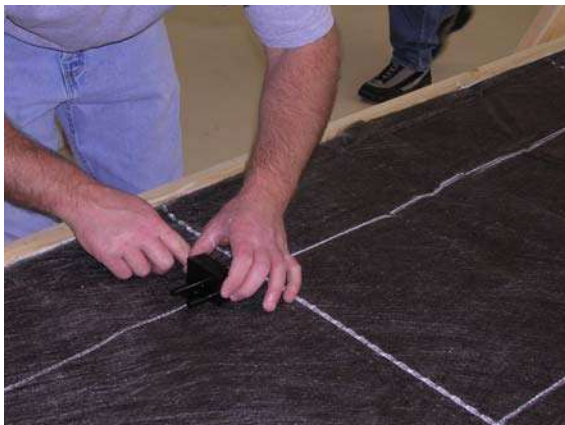
Figure 20: Marking sensor contact points
