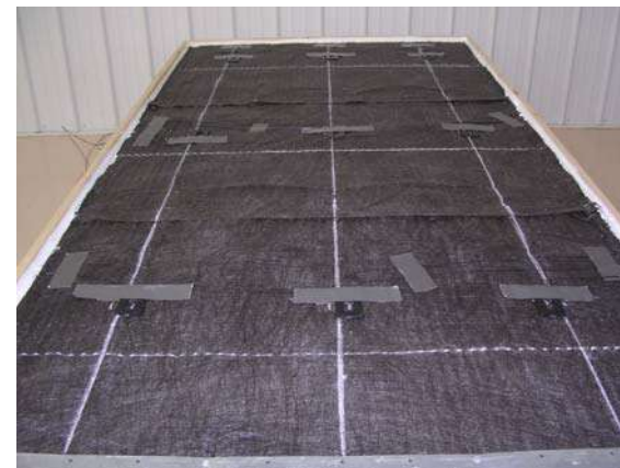
Figure 23: Sure Cavity layer completed
