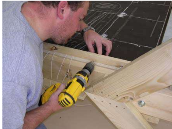
Figure 13: Drilling sensor wire guide holes
