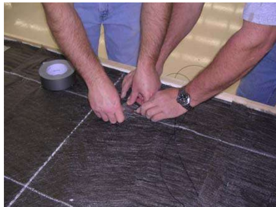
Figure 21: Securing sensor wires
