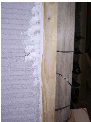
Figure 38: Sealed mortar edge
