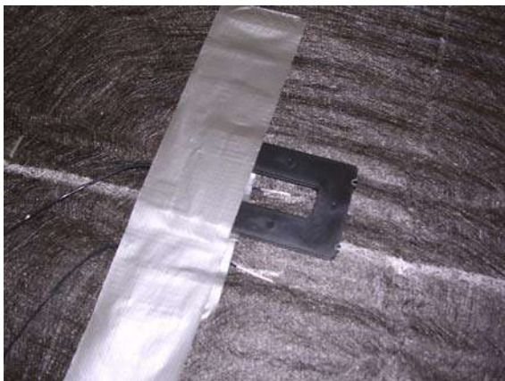
Figure 22: Sensor contact points with shim
