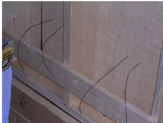
Figure 4: Plywood Layer sensor wires, rear view
