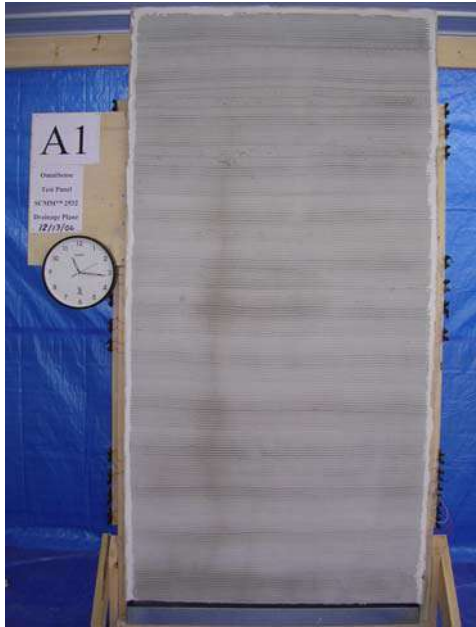
Figure 44: Panel A surface, 21 hours after spray application #1
