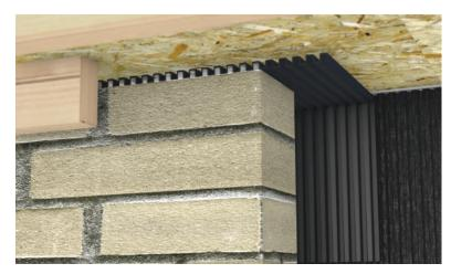
Floor Edging can be used in brick & stone soffit details to vent the rainscreen air gap
