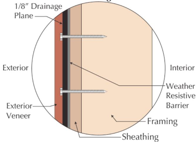
**Screw Fasteners With Rigid Boardstock Insulation
