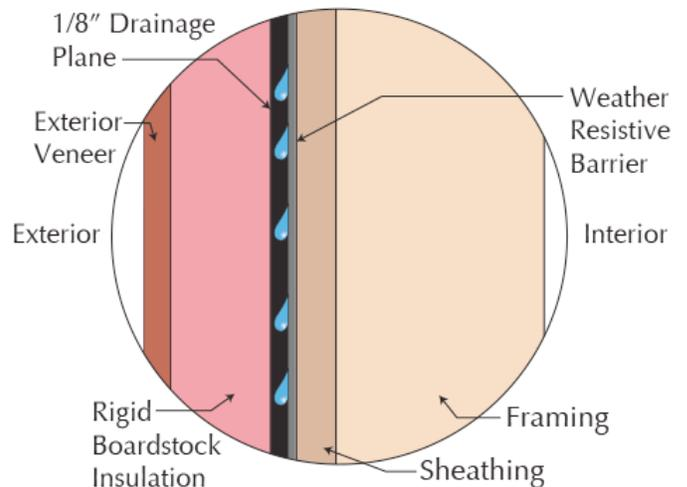
**Drainage Plane with Weep Detail
