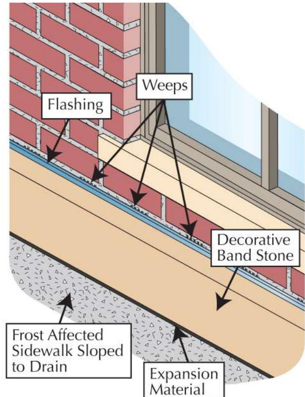
Risk Zones #9 and #10 are the two on-grade details that contact the bottom perimeter of the building on each side of the front stoop. (See Sample Building and Details 9 and 10) The grade surface on Detail 9 is a frost-affected sidewalk; the grade surface on Detail 10 is landscaping stone.
