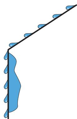
it can be a very concentrated flow. When it lands on a lower surface, it can, over time, erode the lower construction detail. The roof run-off water from a higher roof delivered in a slow "drip, drip" fashion, creates a perpetually wet condition for the lower construction detail. This perpetually wet state is extremely undesirable from a moisture management standpoint. (H & I)
