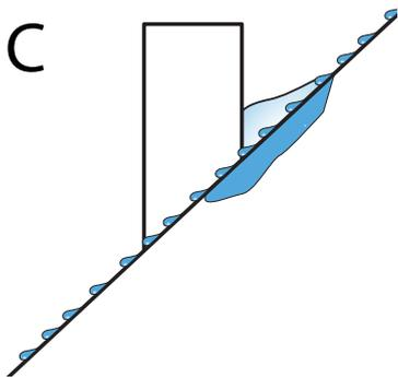
We should also reduce the number of projections or obstructions that are in the path of this draining liquid water. Anything that slows the flow of liquid water off of a construction detail such as chimneys or vent stacks increases the amount of time that liquid water will spend on the construction detail. (C)
