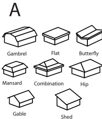
The roof style depends on numerous factors including architectural style, distance to be covered, budget, etc. Generally, for moisture management purposes, the more slope the better.
