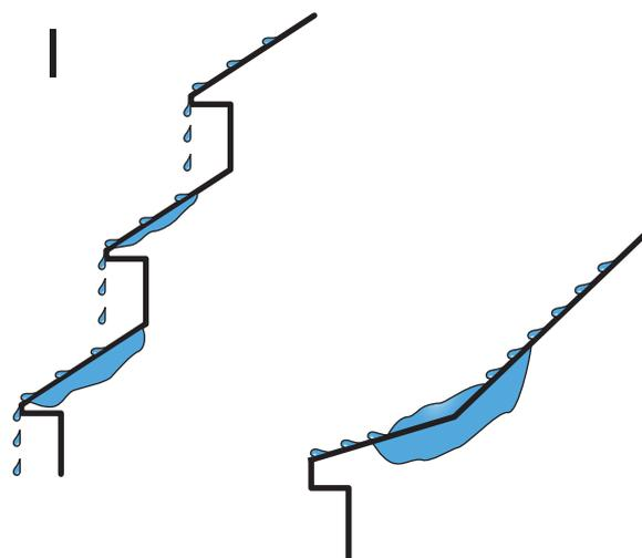
grow a very healthy crop of mold that is hazardous to the health of the building's occupants. Designing a construction detail that allows the moisture that enters it to have a designed way to exit it is probably a good idea. (J & J-1) In fact getting moisture "out of" a construction detail is the "Law!" (2009 IBC R703.12.1.)
