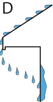
Once the water reaches the roof perimeter, where does it go? (C-1) A good rule to follow is to not allow it to come back into contact with the building or any other construction detail. (D) There should be a relationship between the depth of the overhang (eave) and the height of the wall from eave to grade. (E) This ratio is valid only up to a certain height.
