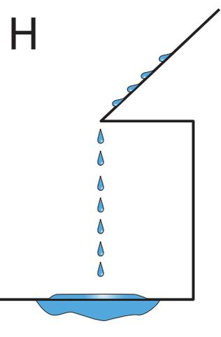
into the construction detail. If liquid water flows from one roof to another and then another, moisture management becomes extremely difficult if not impossible.
