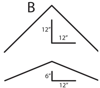
The greater the slope (pitch) on a roof, the faster liquid water can run off. (B) This is important because the less time liquid water is on a construction detail (roof) the less the likelihood it will absorb into that construction detail.
